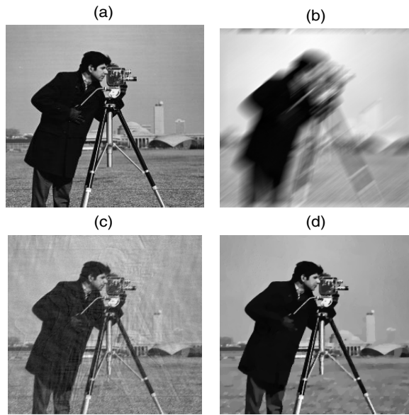
Figure 4. Restoration of the 256 \times 256 Cameraman image blurred by motion: (a) original images; (b) images blurred by motion and noise; (c) restoration by algorithm 2.1 with \Theta = \Theta_0 ; (d) restoration by algorithm 2.1 with \Theta = \Theta_1 .
